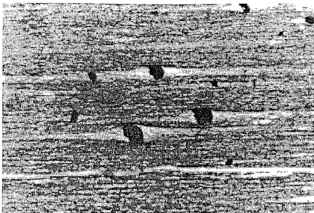
Figure 3b. Microscopic view of structural fabric in the Ninemile fault zone. The section is cut parallel to the lineation but perpendicular to the foliation. The asymmetric pressure shadows (white) around the pyrite grains (black) indicate normal-slip motion along the Ninemile fault.
